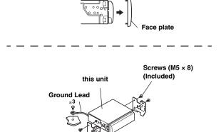
Secure the ground lead of the unit to a clean metal spot using a screw
